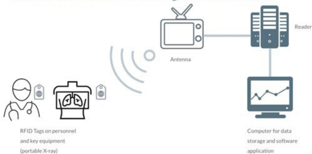
Figure 1 RFID system infrastructure. RFID, radiofrequency identification.
